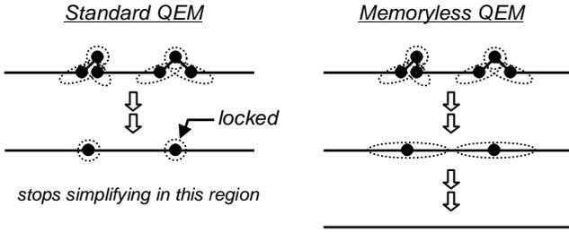
Figure 6: Illustration of standard QEM and memoryless QEM simplification. The dashed ovals symbolize the shapes of the quadric functionals  $Q_p^v$ ; (a) in the standard scheme they are computed once in a preprocess and subsequently summed during simplification; (b) in the memoryless scheme they are computed using the mesh simplified so far.
