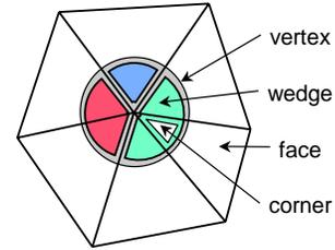
Figure 4: Wedge-based mesh representation.
