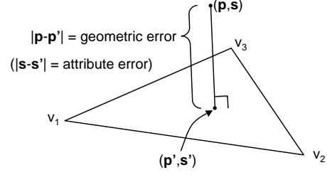
Figure 2: Correspondence between point  $\mathbf{p}$  with attribute  $\mathbf{s}$  and its projection onto the plane spanning face  $(v_1, v_2, v_3)$ .
