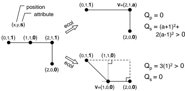
Figure 7: For a polygonal curve in  $\mathbf{R}^2$ , illustration of trade-off between geometric accuracy ( $Q_p = 0$ ) and attribute accuracy ( $Q_s = 0$ ). Attribute accuracy can cause bias towards the center of curvature when the attribute gradient is high.
