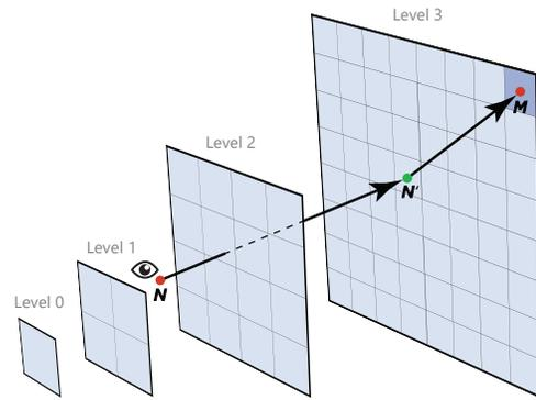
Fig. 13. Hierarchical tiling structure and priority computation. The arrows depict the distance used for priority computation in level-of-detail ( $z$ ) and spatially ( $x, y$ ) between the viewport centered at  $N$  and a tile  $M$ .
