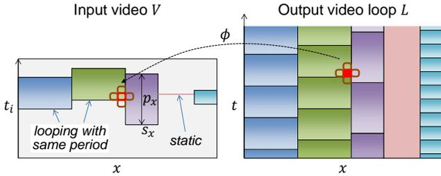
Fig. 6. A video loop  $L$  is formed from an input video  $V$  by repeating some temporal interval at each pixel  $x$  using a time-mapping function  $\phi$ , specified using a period  $p_x$  and start frame  $s_x$ . The consistency objective is that for any output pixel color (shown in solid red), its spatiotemporal neighbors should have the same values as the corresponding neighbors in the input [Liao et al. 2013].
