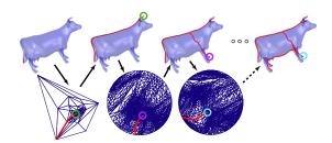
**Figure 1:** Iterative Cutting Algorithm. We start a short cut. The resulting parametrization has high distortion at the center. The worst undersampled area is near the horns. We then cut, and reparametrize. We stop when adding a new cut increases the average distortion or undersampling.
