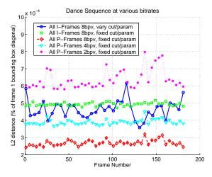
**Figure 7:** Dance sequence (7061 vertices) encoded: at 8 bits per vertex (bpv) using a customized cut and parametrization per frame (vary); at 8 bpv using Geometry Images using only I-Frames; and at 8,4 and 2 bpv using P-Frames (0.3 size ratio between P-Frames and I-Frames). Notice that the encoding using P-frames at 4 bpv is better to using only I-frames at 8bpv.
