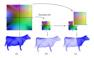
**Figure 10:** Level-of-Detail: by decimating the geometry image (a) we obtain a lower resolution version (b); We can combine the two to support a multi-resolution version of the mesh (c); care must be taken at the transition edges, this is a simple operation due to the regularity of the mesh.
