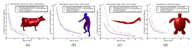
Figure 3: Rate Distortion Curves: comparing Geometry Images to Touma/Gostman (TG) encoder, and Spectral Compression
