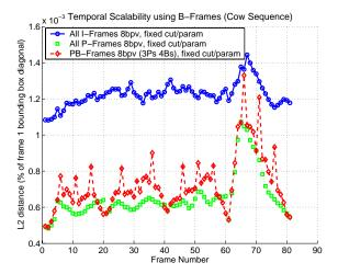
**Figure 6:** The use of B-frames allows the decoder to skip them if necessary. One simple way to implement temporal scalability is by introducing B-Frames. The animation can be played at half the frame rate just by dropping the B-Frames.
