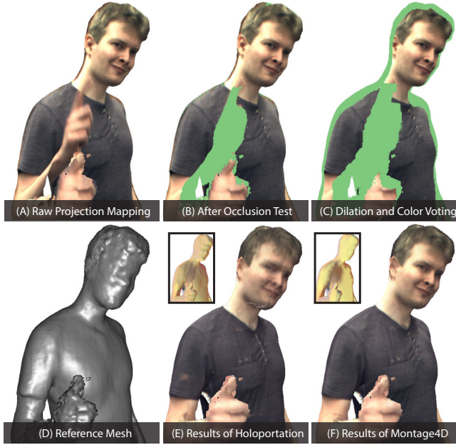
Figure 3: This figure shows how texture weight fields improve the rendering quality compared to the baseline approach. Holoportation removes several ghosting artifacts by taking advantage of dilated depth maps and majority voting algorithm (top row), however, the rendering still suffers from fuzziness and visible seams (bottom row). (A) shows the raw projection mapping result from an input video texture, (B) shows the culling result after the occlusion test, (C) shows the culling result after using dilated depth maps and majority voting algorithm, (D) shows the input mesh, (E) and (F) respectively shows the rendering results from the baseline approach and our algorithm, together with the corresponding texture weight fields for comparison.
